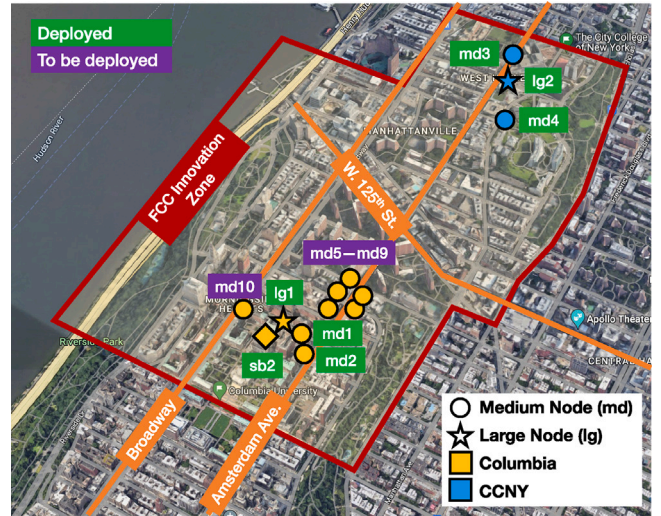
Fig. 8. Location of the deployed COSMOS Sandbox2 (sb2), two large nodes (lg1–lg2), and four medium nodes (md1–md4) within an FCC Innovation Zone in West Harlem, NYC, with six more medium nodes (md6–md10) that will be deployed in the future.
